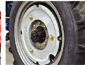
Rear Wheel Track Stepless Adjustable
