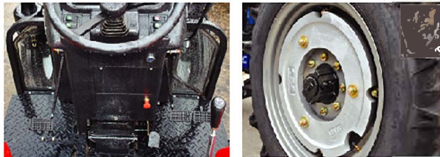
Rear Wheel Track Stepless Adjustable
